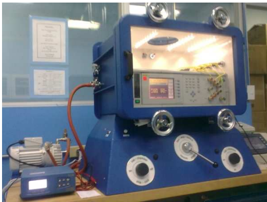
Figure 2. Barometric Chamber with a Thermometric resistance bridge
